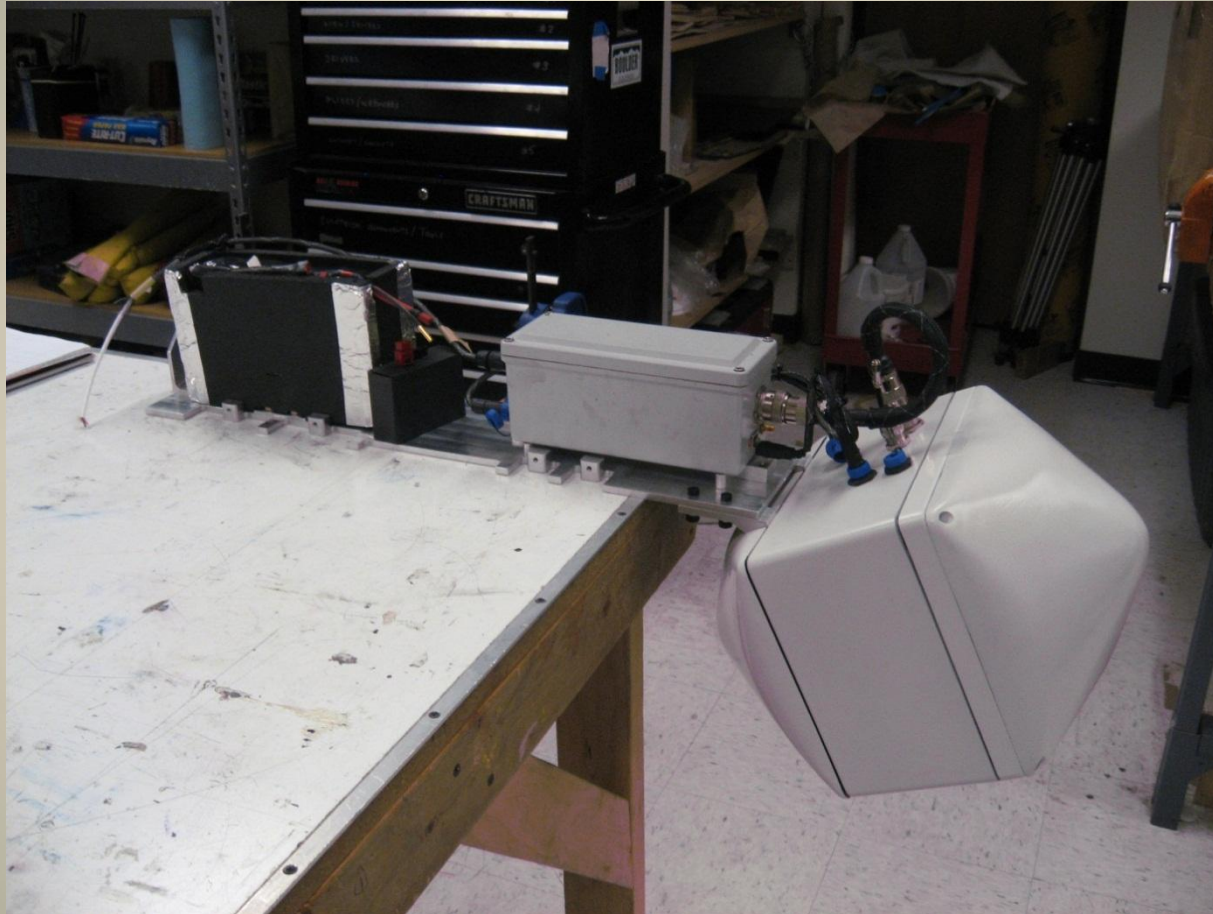
CULPIS-X in CU Lab. Sensor package on right, data acquisition box in middle, battery on left
